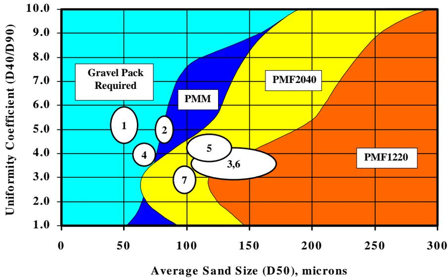
Figure 3: Screen Media Selection Chart for standard non woven screen media: PMM (60  $\mu\text{m}$ ); PMF2040 (120  $\mu\text{m}$ ); PMF1220 (200  $\mu\text{m}$ ). Application to field cases summarized in Table 1.
